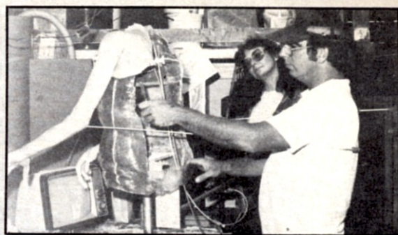
Far Left: Robert Short attaches the latex arms to the plastic "heart-light" chest. Above: Don Pennington and Lucy Seaman adjust the brace that supported E.T.'s mechanical head. Note the thin dowels protruding from the elbows, a muppet-like arm movement. Cables leading out the back of the chest were attached to air bladders, which made the heart pulsate. Left: The completed chest, painted to match the foam latex versions.
